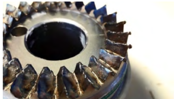
Figure 4. Serration teeth on the impeller for stage 1 (top) and stage 2 (bottom).
